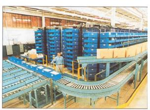
Global's carousel system, consisting of four 10-foot-high strings, has taken over half the operation's volume.
